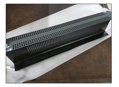
Summary: Drill performed 1500 holes with excellent quality with no delamination nor burs.
