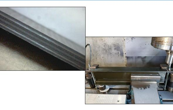
Summary: End-mill ran 100 meters in material with no delamination to the satisfactory of the customer.
